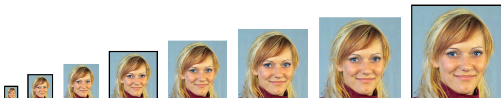
Figure A-3 – Resolution separation in arithmetic progression – Property of DCT based image coding.
